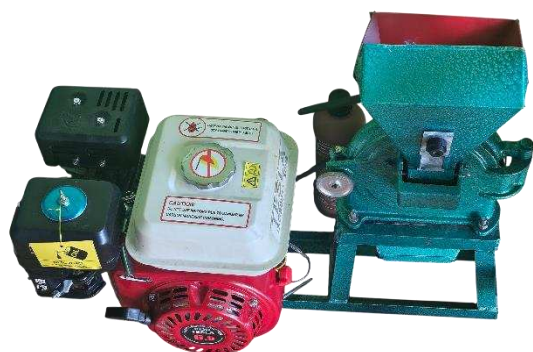
Figure 1. FFC-45 disk mill used for maize flour production during the community service training program
