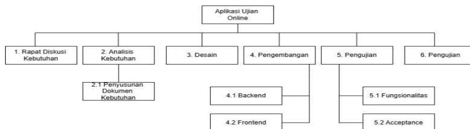
Gambar 2. Web Breakdown Structure (WBS)
