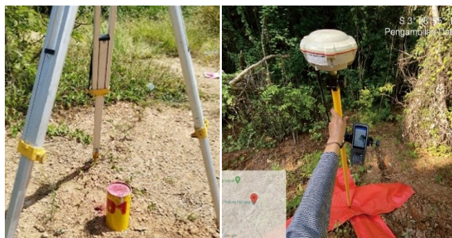
Fig. 2. Establishing benchmarks (BM) and ground control points (GCP) using geodetic GPS for high-precision mapping.
