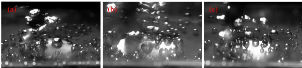
Fig. 10. Surface visualization: (a) test specimen A at \dot{q} = 21.53 \text{ kW/m}^2 , (b) test specimen B at \dot{q} = 25.61 \text{ kW/m}^2 , and (c) test specimen C at \dot{q} = 27.36 \text{ kW/m}^2
