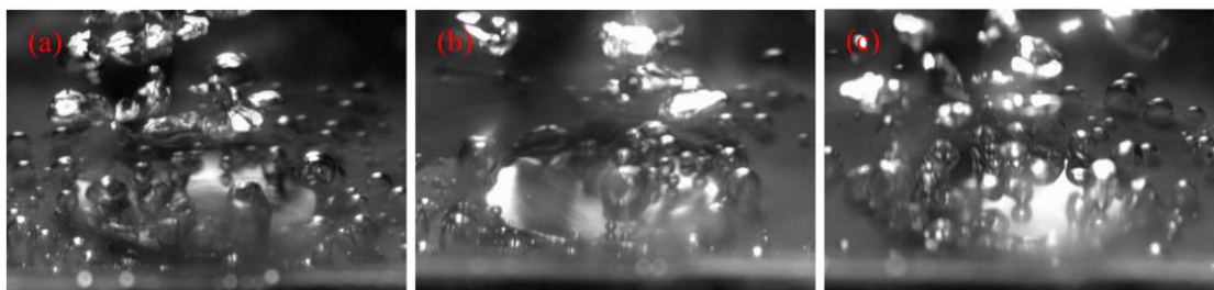
Fig. 11. Surface visualization: (a) test specimen A at \dot{q} = 37.19 \text{ kW/m}^2 , (b) test specimen B at \dot{q} = 39.89 \text{ kW/m}^2 , and (c) test specimen C at \dot{q} = 37.03 \text{ kW/m}^2
