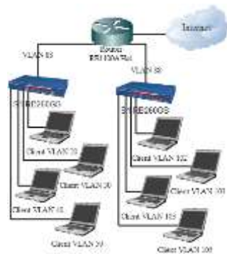
Gambar 5. Rancangan Topologi Jaringan Inter-Vlan Routing
