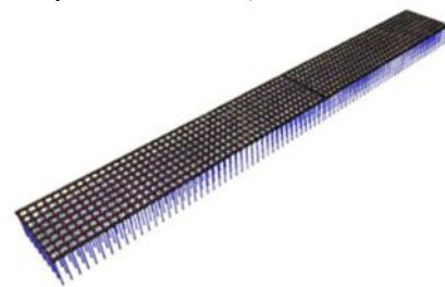
Gambar 1. Model 3D - Deck-on-pile Interface
