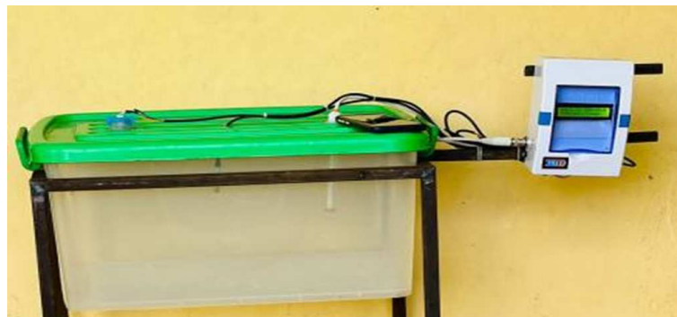
FIGURE 11 An IoT monitoring device with a test container
