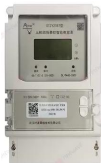
Gambar 7. kWh Advanced Metering Infrastructure (AMI)
