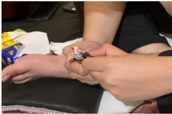
Figure 4. Testing DS18B20 Sensor with Heat Source
