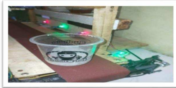
Gambar 7 Proses Gelas Cup Terdeteksi Sensor Photodioda 1
