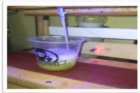
Gambar 10 Proses Gelas Cup Terdeteksi Sensor Photodioda 4
