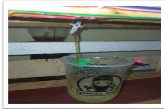
Gambar 9 Proses Gelas Cup Terdeteksi Sensor Photodioda 3
