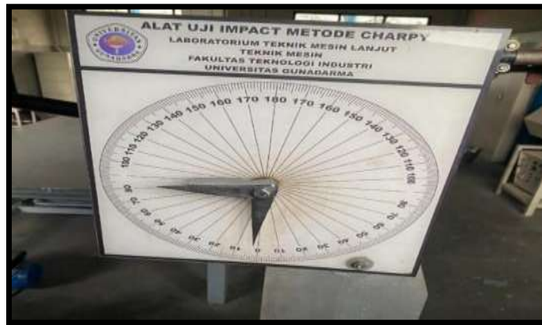
Gambar 13 Proses Pengujian Impact Charpy
