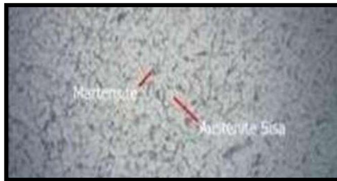
Gambar 17 Struktur mikro proses Quenching Suhu Ruang
