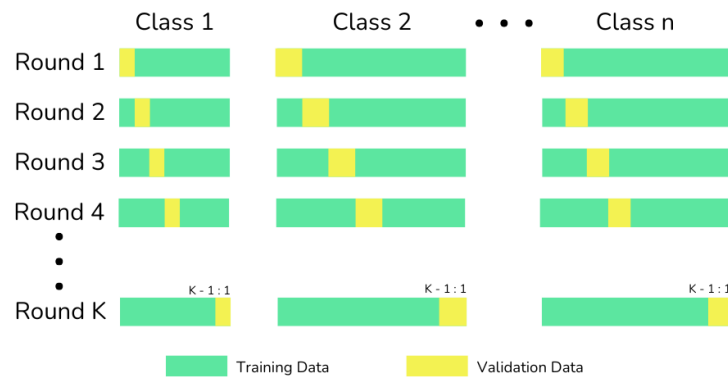
Fig. 2. Schematic Diagram of Stratified K-fold Cross Validation
