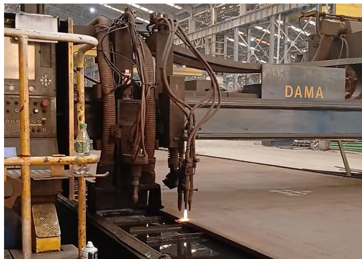
Gambar 3. Mesin CNC cutting plasma di PT. Kenertec Power System
