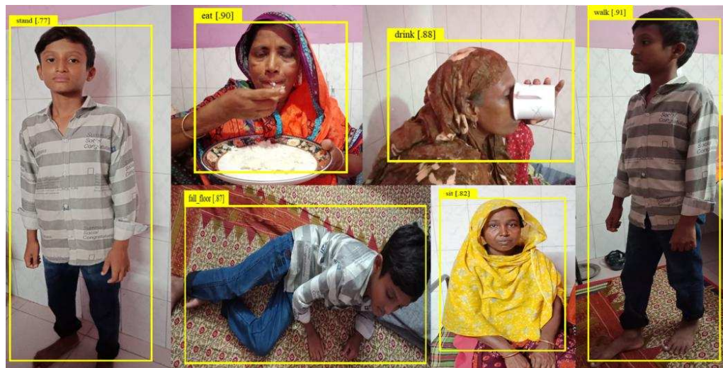
Figure 8. Performance on the real-time testing with testing accuracy score left: “stand”, middle: “eat”, “drink”, “fall_floor”, “sit” and right: “walk”
