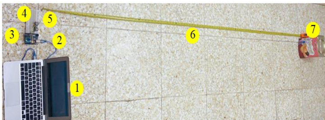
(1) Laptop. (2) Arduino cable. (3) Arduino Uno. (4) Breadbord. (5) Ultrasonic sensor. (6) measuring tape tool. (7) Object.
