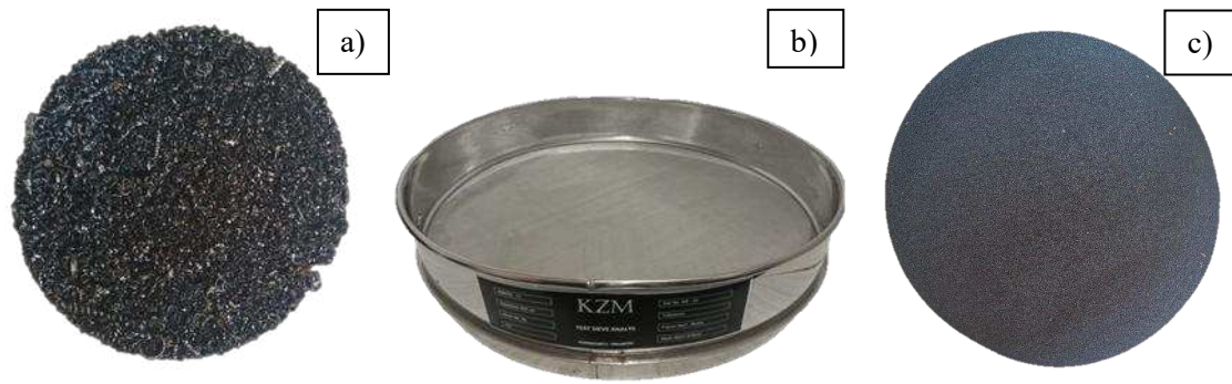
Figure 2. a) Machining waste, b) Test sieve mesh 100, c) Powder after sieving.
