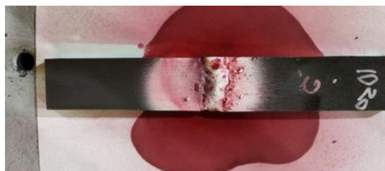
Figure 3. Results of red dye penetrant testing
