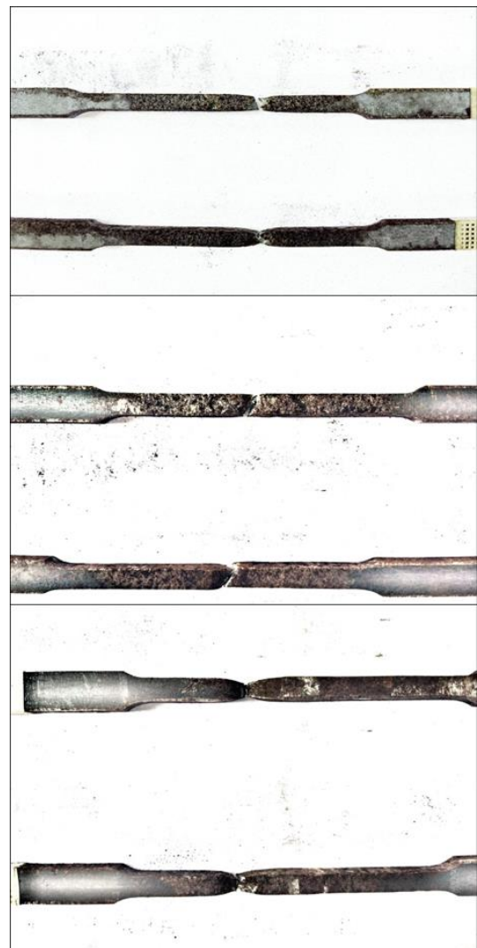
Figure 9. Variations in welding speeds of 5, 10, and 15 m/min on AISI 1020 and AISI 1050 steel after tensile testing
