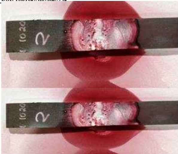
Figure 4. Data from observations using red dye penetrant on tensile test specimens
