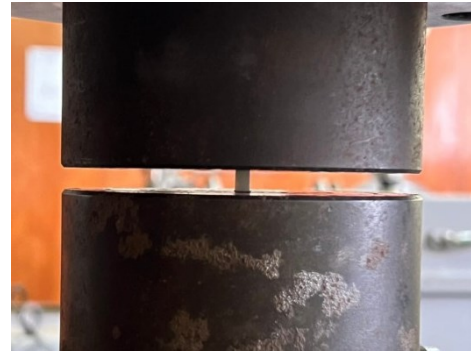
Figure 4. The specimen was tested for compression strength with a universal testing machine
