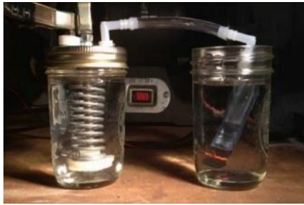
Gambar 2. Generator oxyhydrogen tipe wet cell (Anon., n.d.)
