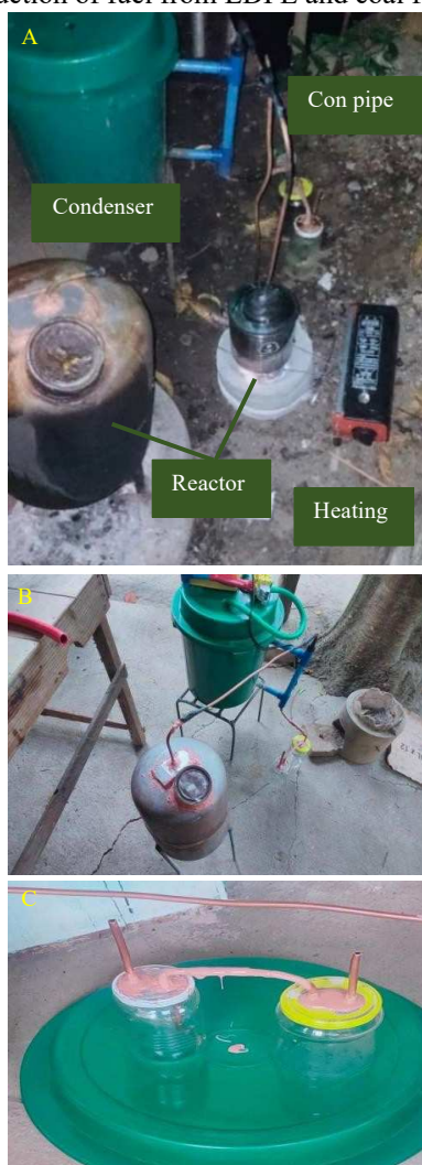
Figure 5 Experimental setup for production of fuel from LDPE: (A) Parts of the experimental setup, (B) Condenser and reactor, and (C) One-way valve and gas chamber
