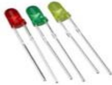
Gambar 6. Light Emitting Diode [17]
