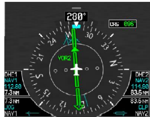
Gambar 17A Instrumen HSI GIFD Trainer CLP
