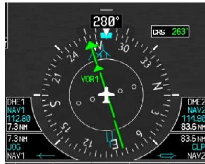
Gambar 16 A. Instrumen HSI GIFD Trainer JOG
